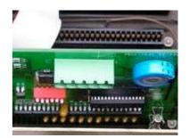
If a scoring system with standard APS is connected (Qubica, Steltronic, MaxS ...) dipswitch 6 must be in off position. To use the Qubica fast strike signal, the normally closed contact from the F-Box must be connected to pin 3 and 5 with dipswitch 6 in on position.
